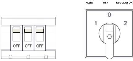
Input and Bypass breakers are OFF.
