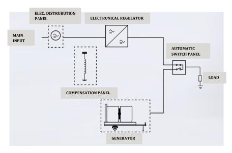
Recommended connections of MRG/MST33 Series Static Voltage Regulator
