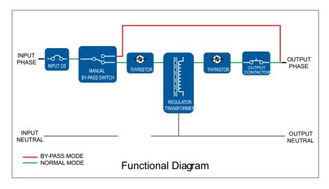
MRG/MST33 Series Static Voltage Regulator Functional Diagram
