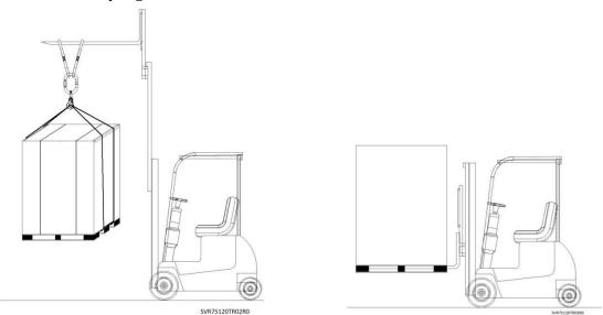
The regulator device shipment must be done on pallets.
